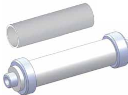
Filter element on filter holder
