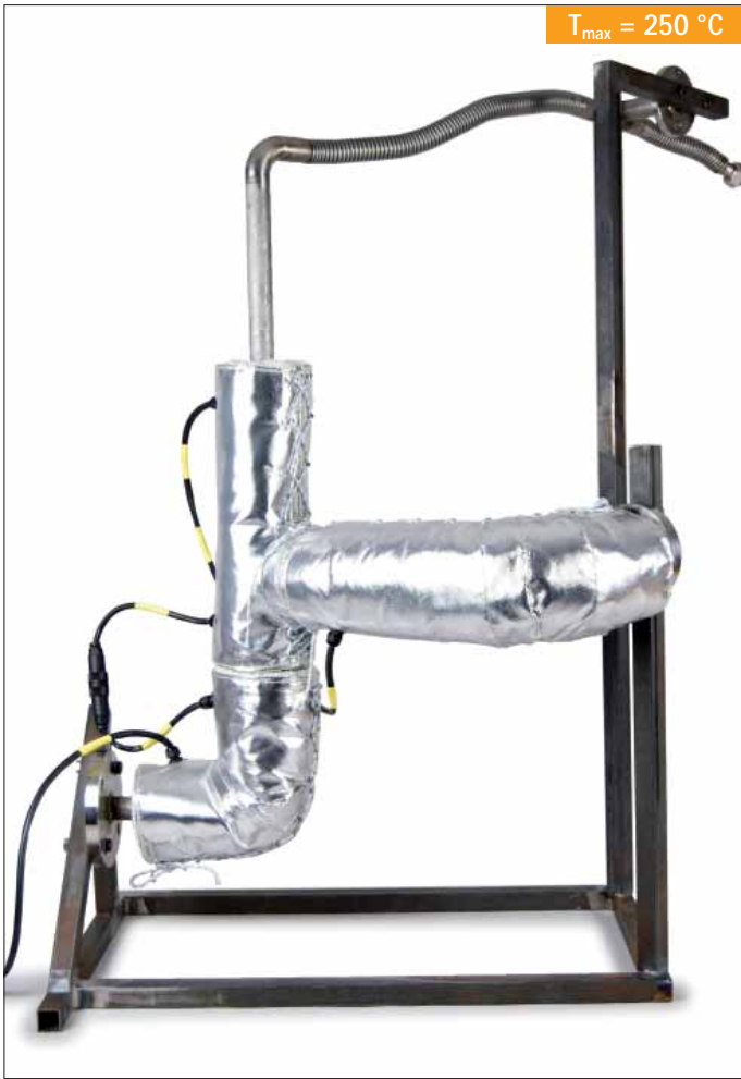
Types WOG – Heating jacket for measuring equipment
