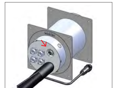
4. Unneeded inlets are closed with blind plugs
